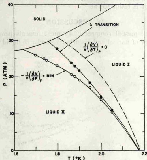
FIG. 7. Phase diagram of He<sup>4</sup> showing the melting curve, the  $\lambda$  line, the locus of zero expansion coefficient, and the locus of minimum in compressibility.
