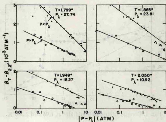
FIG. 8.  $\beta_T - \beta_{2.2}$  versus  $\log|P - P_\lambda|$  for liquid He<sup>4</sup> at several temperatures. The upper curve is for  $P < P_\lambda$  and the lower curve is for  $P > P_\lambda$  at each  $T$ .
