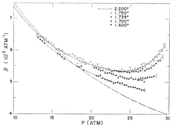
FIG. 6. Compressibility of liquid He<sup>4</sup> at several temperatures below 1.76 and at 2.200°K.
